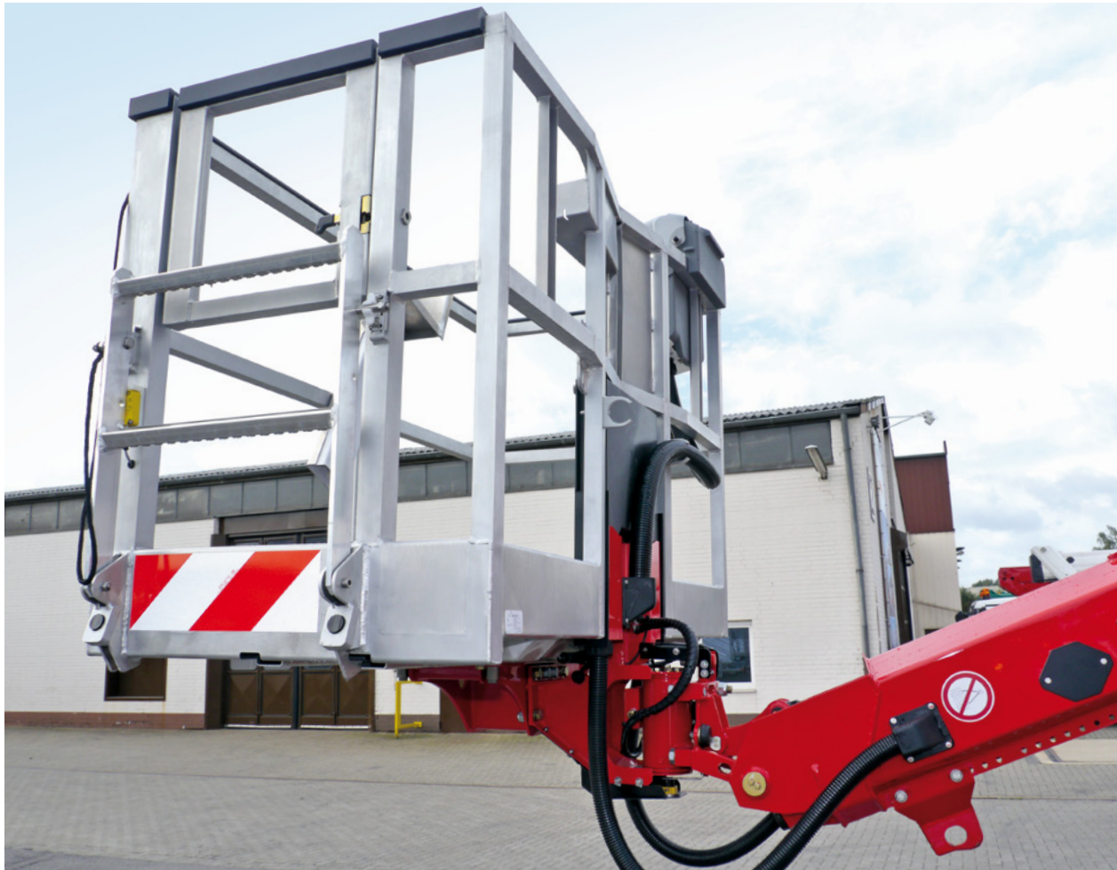
The angle sensor underneath the working cage measures the swivel angle of the cage
